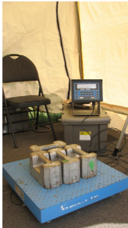
Figure 5. Scale checking using a calibration weight set.
